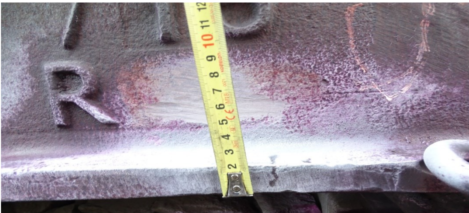
Transverse cracks on the casting Defect code 724N
